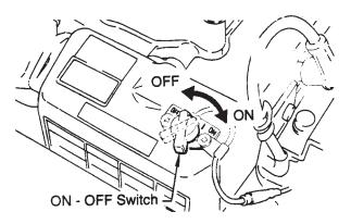
Figure 8. On/Off Switch
